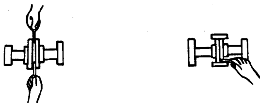
Figure 3B. Aligning Non-Spider Type Couplings
