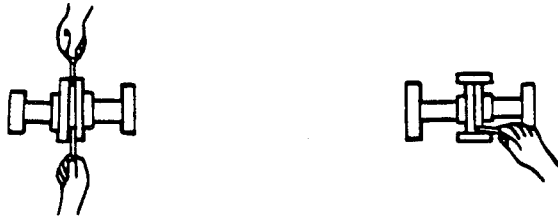
Figure 3B. Aligning Non-Spider Type Couplings
