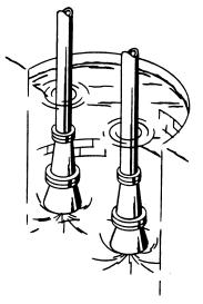
Figure 3. Using Two Pumps in the Same Sump
