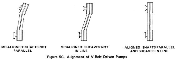
Tighten the belts in accordance with the belt manufacturer's instructions. The belts will slip if they are too loose; there will be excessive power loss and possible bearing failure if they are too tight. Select pulleys that will provide the proper speed ratio. Overspeeding the pump may damage both pump and driver.
