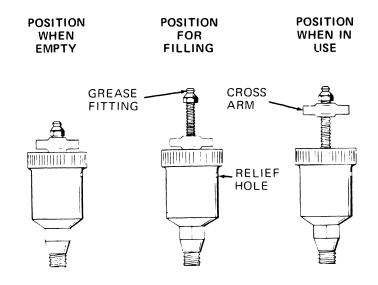
Figure 3. Automatic Lubricating Grease Cup
