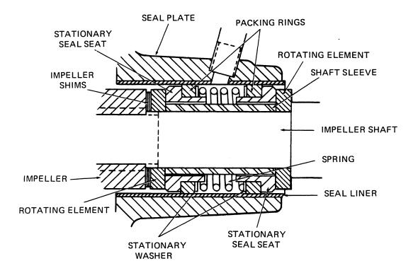
Figure 2. GS-750 Seal Assembly
