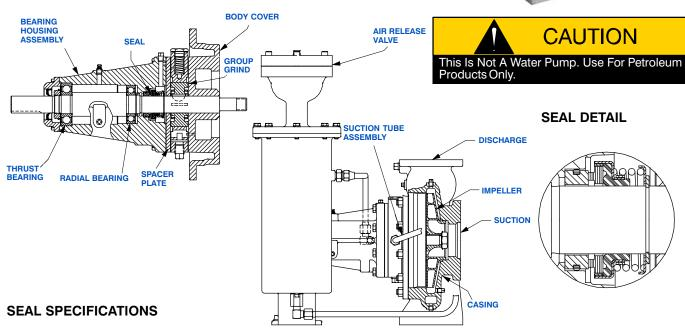
Seal: Mechanical; Self-Lubricated. Fluorocarbon Elastomers (DuPont Viton® or Equivalent). Carbon Rotating Face; Ni-Resist Stationary Face; Maximum Temperature of Liquid Pumped is 160°F (71°C).
