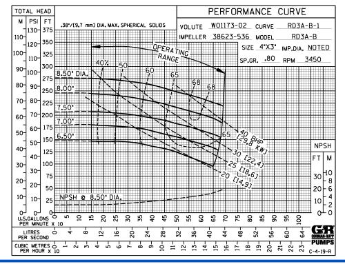
**PERFORMANCE BASED ON PETROLEUM TRIMMED IMPELLER**
