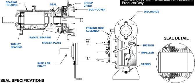
Seal: Mechanical; Self-Lubricated. Fluorocarbon Elastomers (DuPont Viton® or Equivalent). Carbon Rotating Face; Ni-Resist Stationary Face; Maximum Temperature of Liquid Pumped is 160°F (71°C).\*
